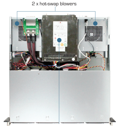
Hot-swap 500W 12V high-efficiency redundant power supply module
